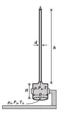
Q.17 When the chimney is closed using a cap at the top, a pressure difference  $\Delta P$  develops between the top and the bottom surfaces of the cap. If the changes in the temperature and density of the hot air, due to the stoppage of air flow, are negligible then the value of  $\Delta P$  is \_\_\_\_\_\_ N m<sup>-2</sup>.
