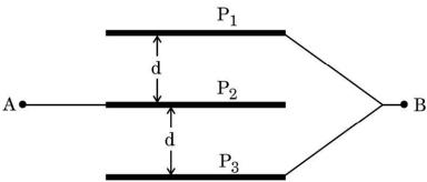
(i) The capacitance of the system between A and B will be:
