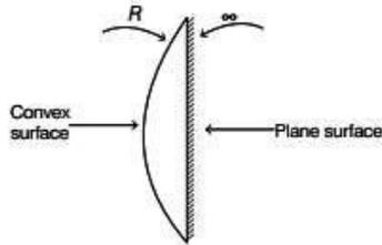
where,  $R_1$  is the radius of curvature of convex surface and  $R_2$  is the radius of curvature of plane surface ( $R_2 = \infty$ ).
