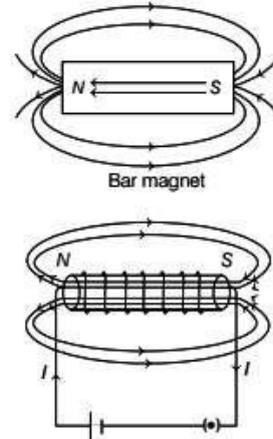
Hence, A bar magnet is equivalent to a solenoid carrying current.
