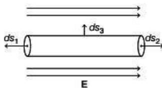
Let  $\phi_1$  and  $\phi_2$  be the flux coming out of a circular cross-sectional surface.  $\phi_3$  is flux through the curved surface. Since, normal to a curved surface is always  $90^\circ$  to electric field  $E$ , so
