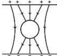
Negative charge would be induced on the upper surface of the sphere and similarly positive charge would be induced on lower surface of the sphere.
