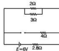
Thus, current in the  $4\Omega$  resistor is zero.  $2\Omega$  and  $3\Omega$  resistors are parallel to each other. Thus, the resistance in the upper branch is given by
