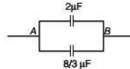
Now,  $C_1$  and  $C_2$  are connected in parallel combination. Hence, equivalent capacitance is given by
