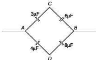
In the upper arm capacitors  $3\mu\text{F}$  and  $6\mu\text{F}$  are connected in series and similarly in lower arm capacitors  $4\mu\text{F}$  and  $8\mu\text{F}$  are connected in series. The equivalent capacitance is given by
