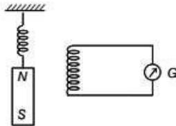
As the emf is induced in the coil eddy currents are also induced in the magnet, which lowers down the total magnetic strength of the magnet. Due to this reason, the magnetic flux linked with the coil decrease and hence amplitude of the deflections produced in the galvanometer also decreases.
