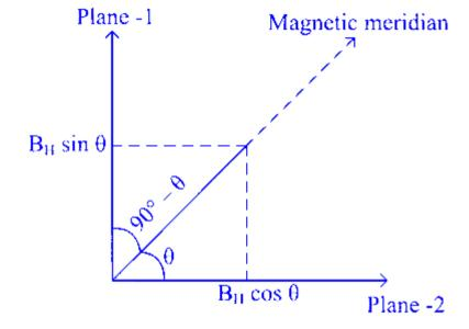
Let plane - 1 and 2 be mutually perpendicular planes makings angle  $\theta$  and  $(90^{\circ} - \theta)$  with magnetic meridian. The vertical component of the earth is magnetic field remain same in two plane but effective horizontal components in the two planes is given by
