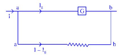
The potential difference,  $V_{ab}=\left(V_{a}-V_{b}
