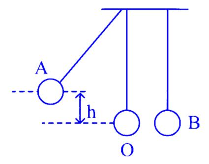
The potential energy of A at height h gets converted into kinetic energy of this mass, at point O, i.e.
