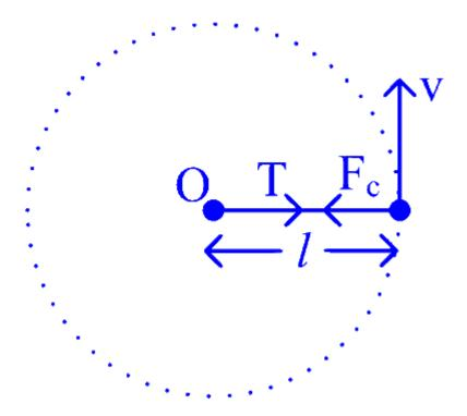
Speed of the particle is v. As, the particle is in uniform circular motion, the net force on the particle must be equal to centripetal force which is provided by the tension (T).
