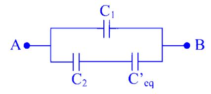
$\because C_1$  is in parallel with the series combination of  $C_2$  and  $C'_{ ext{eq}}$  .
