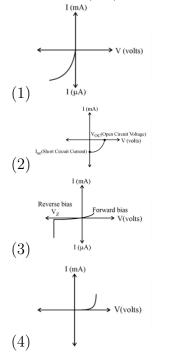
The correct sequence of graphs corresponding to forward biased p-n junction; Zener diode;
