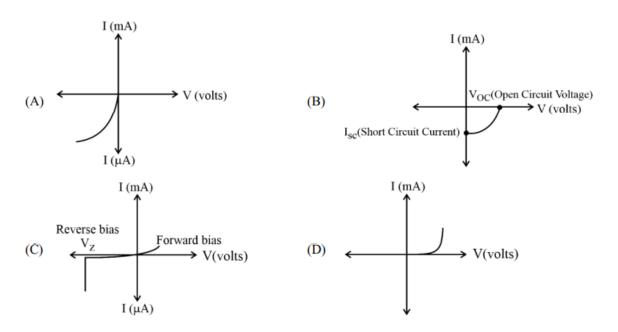
The correct sequence of graphs corresponding to forward biased p-n junction; Zener diode; Photo diode and Solar cell in order is \_\_\_\_\_.
