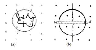
The wire in figure (a) is turning into a circular loop and that in figure (b) into a narrow straight wire. The direction of induced current will be \_\_\_\_\_.
