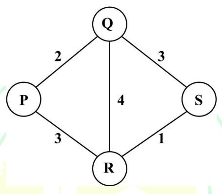
Length of the streets, in km, are shown on the network. The minimum distance travelled by the sweeping machine for completing the job of sweeping all the streets is \_\_\_\_ km. (rounded off to nearest integer)
