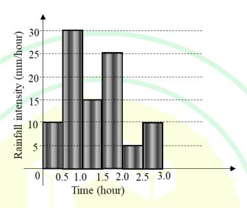
If the storm produced a direct runoff of 12.5 mm, then the  $\phi$ -index of the storm for the catchment is \_\_\_\_\_ mm/hour. (rounded off to two decimal places)
