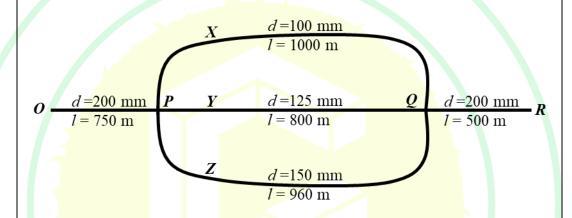
Diameter (d) and length (l) of each pipe are as presented in figure and all pipes are of same material having friction factor (f) of 0.02. Assume acceleration due to gravity (g) as  $10.0 \text{ m/s}^2$ . If the head difference between P and Q is 10 m, then the head loss between Q and R is \_\_\_\_\_\_ m. (rounded off to two decimal places)
