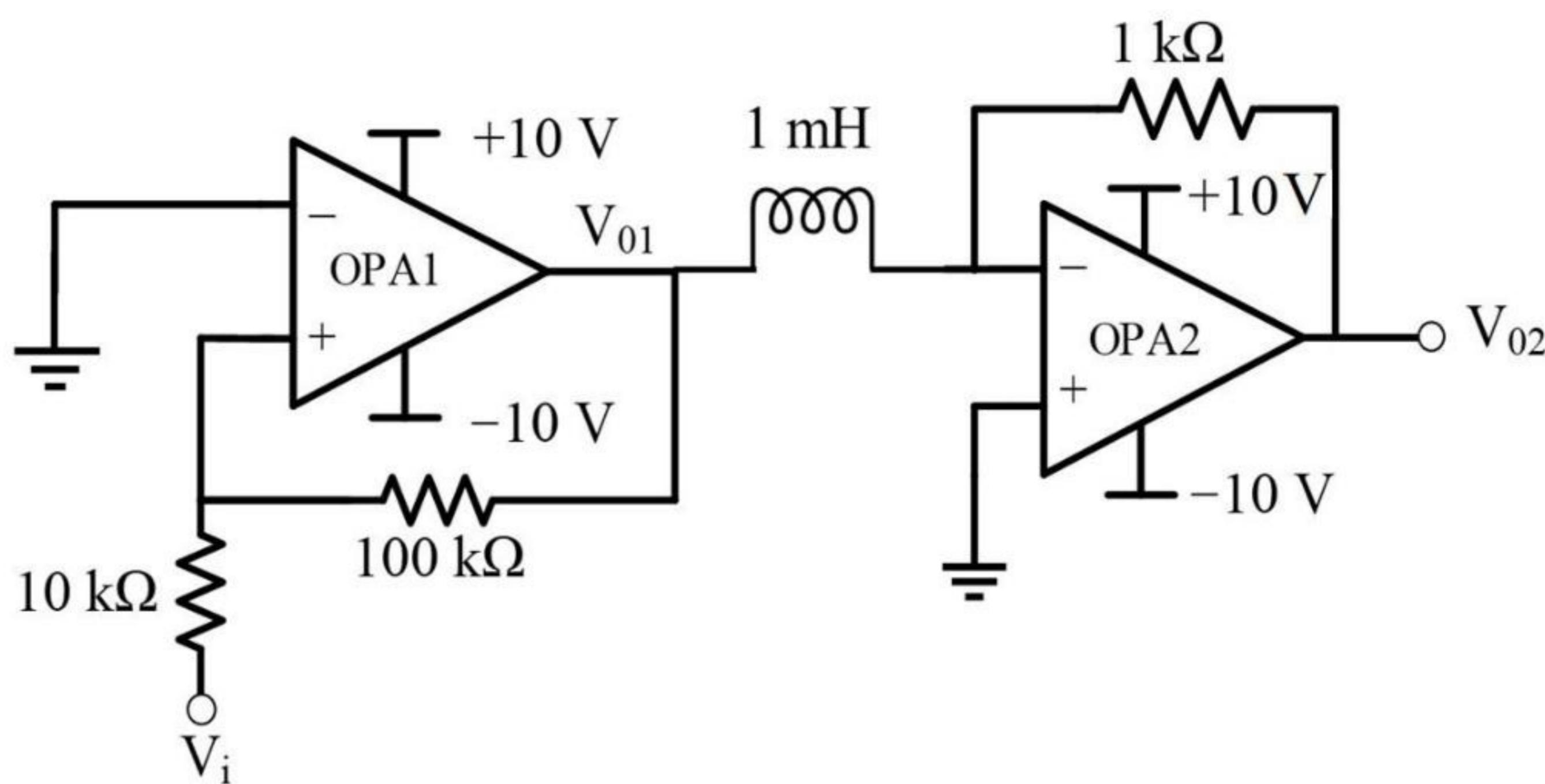
Assume that the initial inductor current is 0 A. The input voltage ( $V_i$ ) is a triangular signal with peak voltages of  $\pm 2$  V and time period of 8  $\mu$ s. Which one of the following statements is true?
