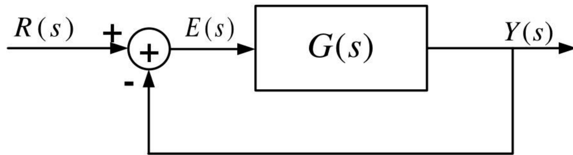
$R(s)$ ,  $Y(s)$ , and  $E(s)$  are the Laplace transforms of  $r(t)$ ,  $y(t)$ , and  $e(t)$ , respectively.
