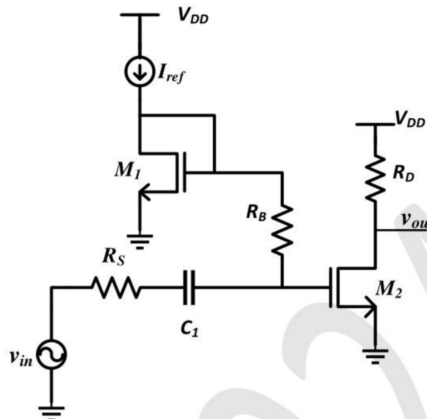
Assuming that capacitor  $C_1$  is a short circuit for AC analysis, the exact magnitude of small signal voltage gain  $\left| \frac{v_{out}}{v_{in}} \right|$  is \_\_\_\_\_.
