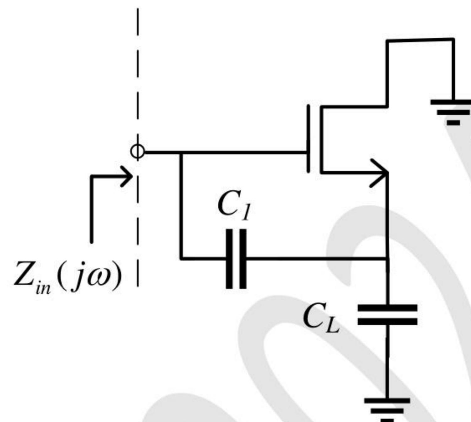
(A)  $\frac{-g_m}{C_1 C_L \omega^2} + \frac{1}{j\omega C_1} + \frac{1}{j\omega C_L}$
