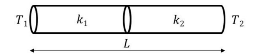
The left and right ends of the connected rod are maintained at temperatures  $T_1$  and  $T_2$  ( $T_1 > T_2$ ). Assume that the rods are insulated from the environment, apart from the two flat ends.
