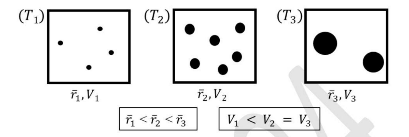
If the cementite in steel is more noble than ferrite, then which one of the three microstructures will have the highest corrosion rate when exposed to an aqueous solution of 3.5 wt. % NaCl?
