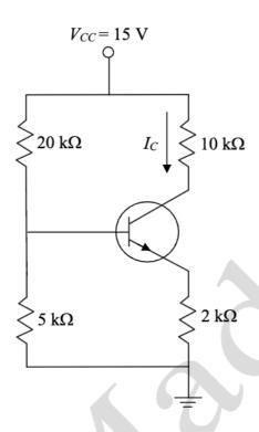
The current  $I_C$  will be \_\_\_\_\_ mA. (Rounded off to two decimal places)
