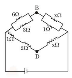
**Solution:** The given circuit is a resistive network. For the potential difference between B and D to be zero, the voltage drop across the resistors must balance out.
