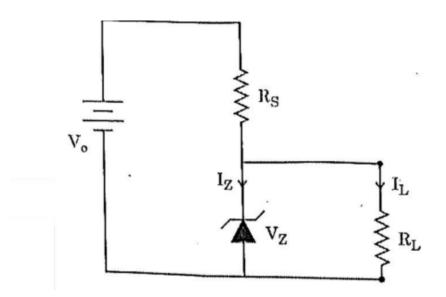
(A)  $V_o = V_z$ (B)  $V_o = V_z - I_L R_L$ (C)  $V_o = V_z$ (D)  $V_o = V_z - I_L R_L$
