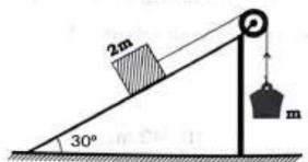
In the adjoining figure, if the pulley and the inclined plane are frictionless, then upward acceleration of the mass m will be
